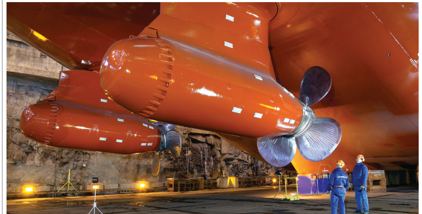
Double Azipod configuration on board Fesco Sakhalin.
